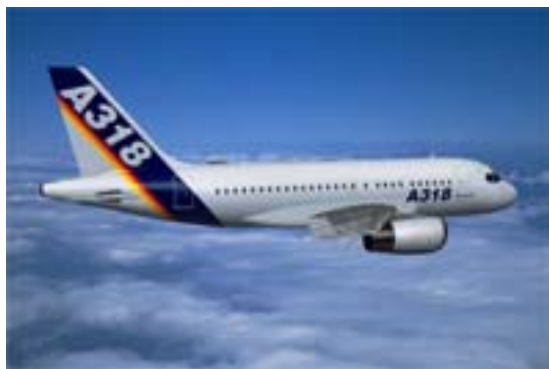
Fig. 5.9: Flying airplane (Airbus A318) as a system with 6 rigid body modes and deformation modes
