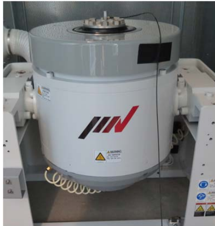
Figure 2: Shaker system i210 (and components) provided by IMV Europe Ltd.
