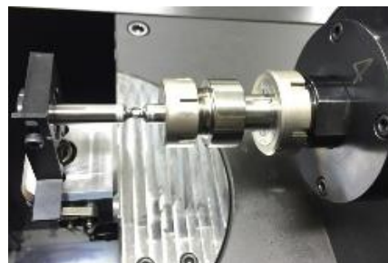
Fig.2: Dual-spindle rotating bending fatigue machine YRB300L (chucking parts and specimen)
