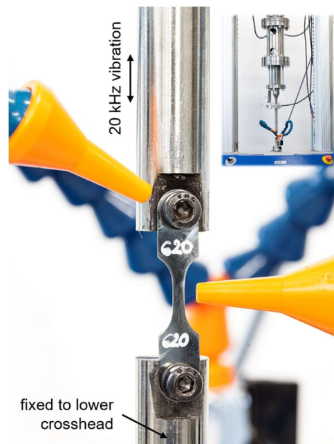
Fig. 2: Overview (top right corner) and detail of the ultrasonic fatigue testing setup at a spindle driven load frame with mounted NiTiNOL specimen
