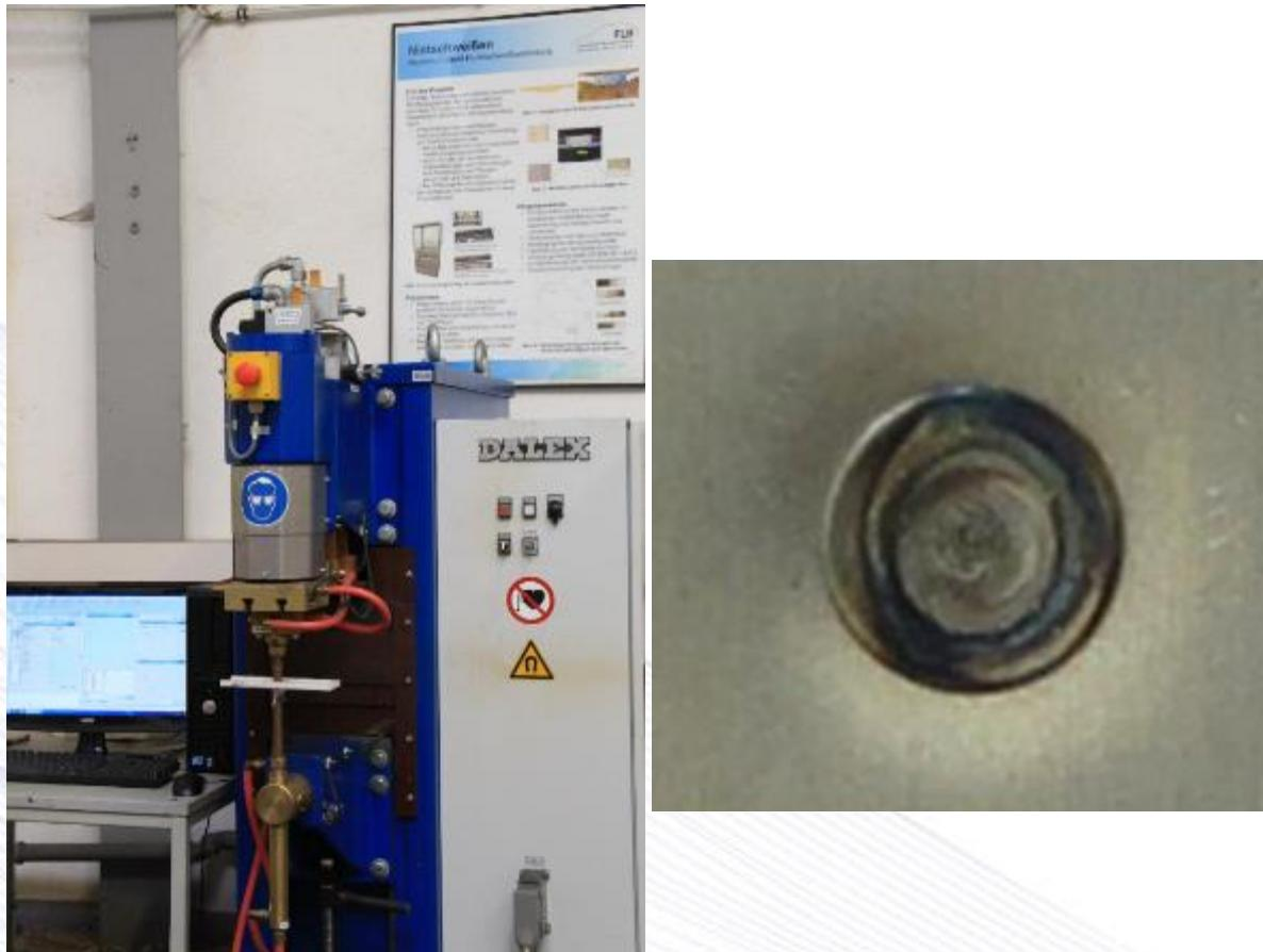
Figure 14: Spot welding system (l.) + novel joining element resistance rivet spot welding (RRSW) (r.)
