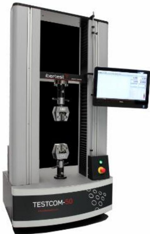
Figure 8: Creep test bench Testcom-50 (Ibertest)
