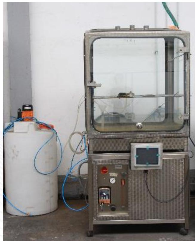
Figure 13:Corrosion chamber with tank (NaCl)
