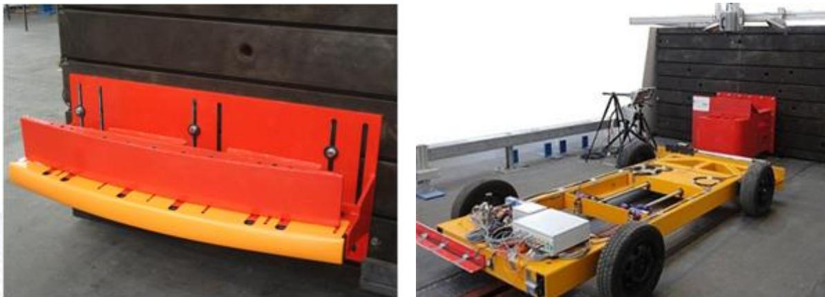
Figure 2: RCAR bumper test barrier (l.) and sledge test setup with 10°RCAR structure test barrier (r.)
