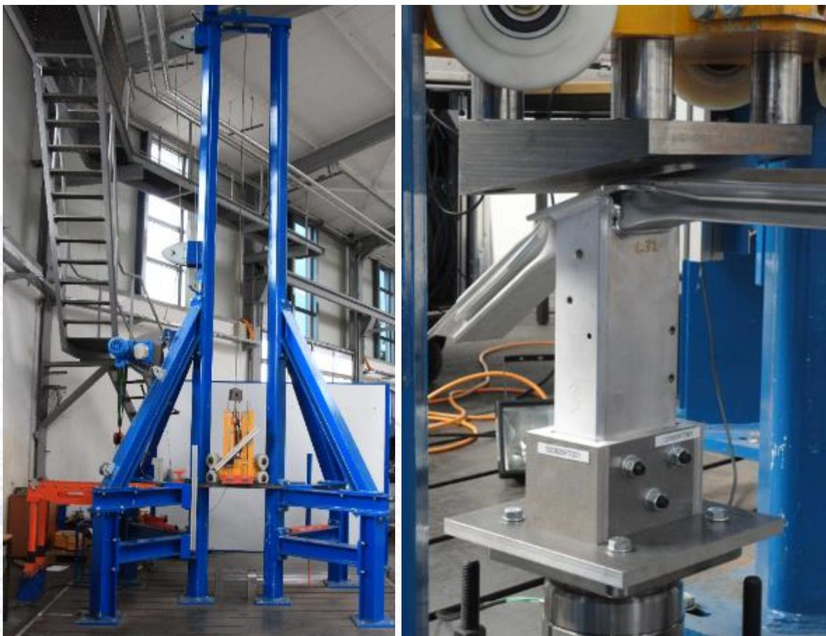
Figure 1: Drop tower (l.) and exemplary test setup of a component test (r.)
