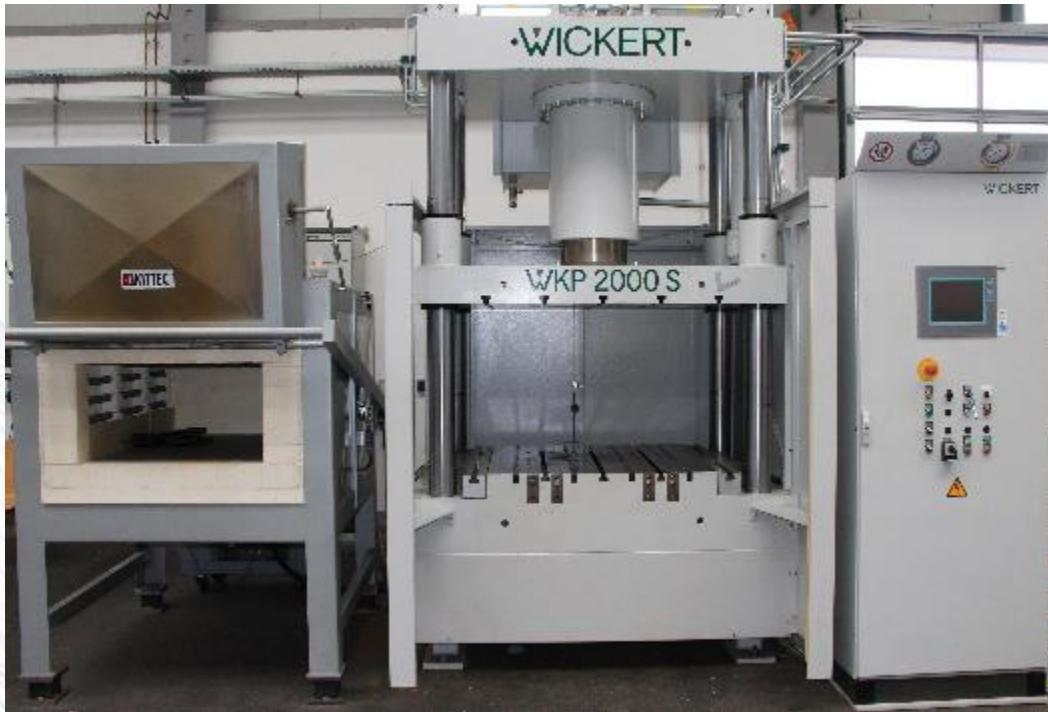
Figure 15: Tempering Furnace (l.) and Hydraulic Press WKP 2000 (r.)
