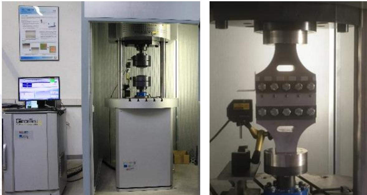
Figure 10: Resonance test bench with test setup for flat specimen (l.) and H-specimen for cyclic testing of joining elements (re.)
