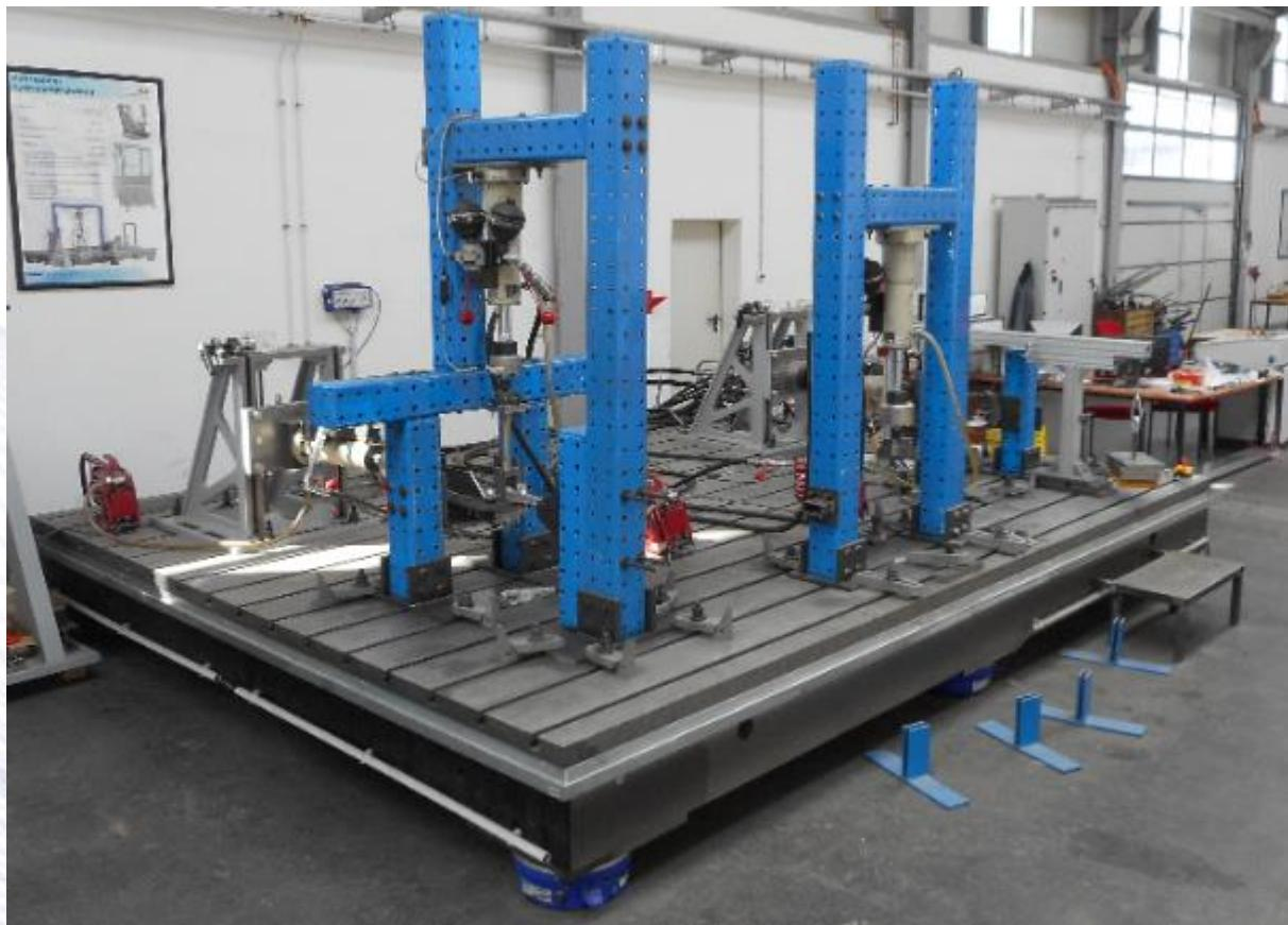
Figure 4: Modular test field for multiaxial component testing
