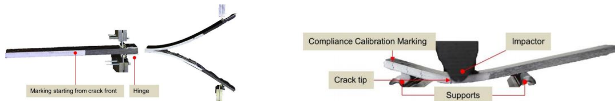
Fig: Shows the test setup for DCB tests (Left) and ENF tests (Right)
