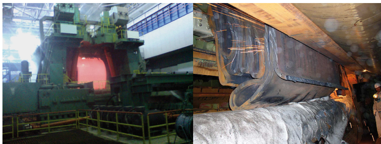
(a) damage by turn-up
