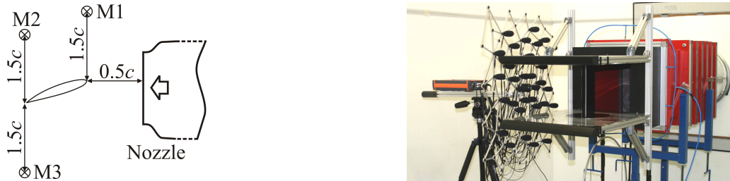
Figure 3. Left: Airfoil section and microphone positions (top view); right: Microphone array next to airfoil
