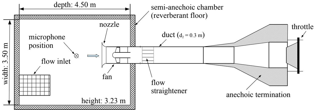
**Figure 2.** Top view of the standardized test rig for acoustic measurements (not to scale).
