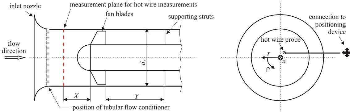
**Figure 3.** Lateral view of the axial fan section investigated (left;  $X = 0.96d_2$ ,  $Y = d_2$ ) and top view (right).
