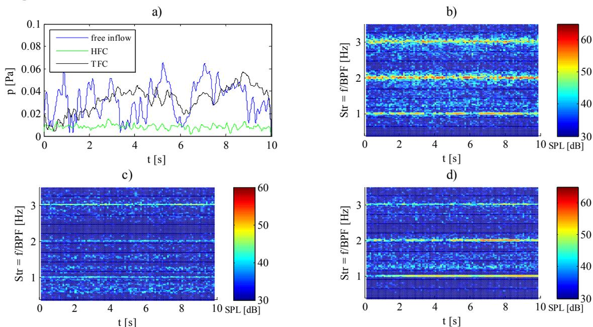
**Figure 5:** Unsteadiness of the acoustic microphone data for different inflow conditions: envelopes of the filtered time signals (a) and spectrograms for the cases of the free inflow (b), HFC (c) and TFC (d).
