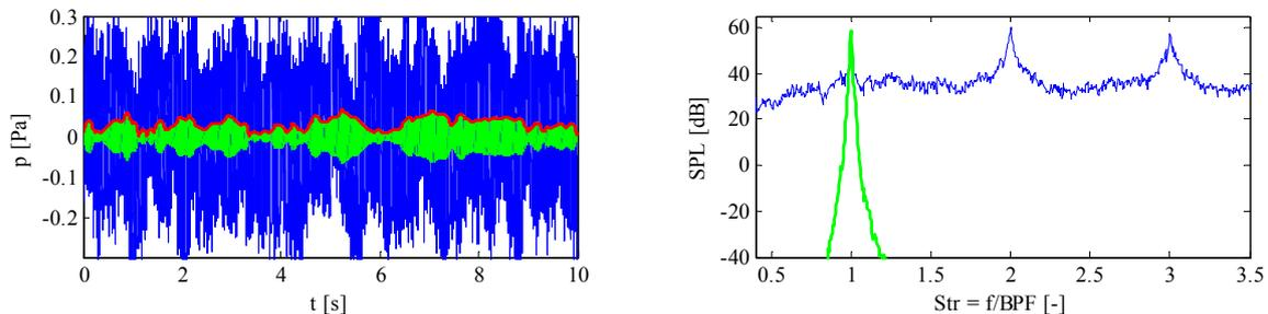
**Figure 4:** Filtered and unfiltered signals of the acoustic microphone data for the case of free inflow in the time (left) and frequency (right) domain: raw signal (—), filtered signal (—), envelope (—).
