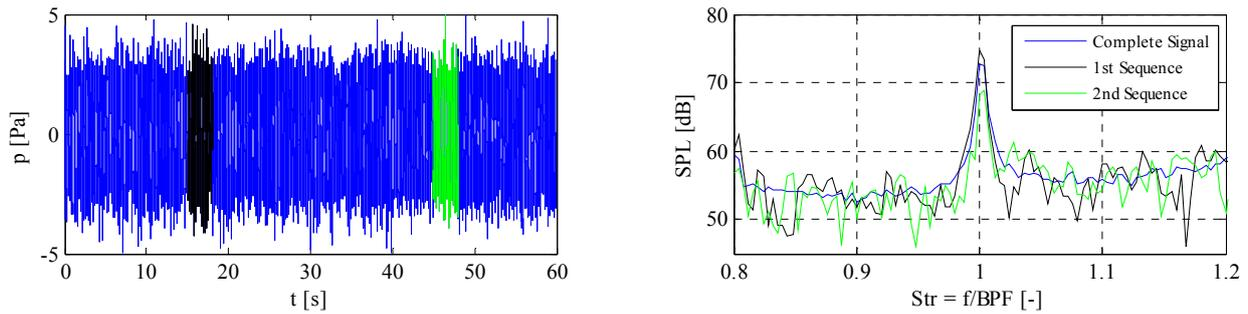
**Figure 1:** Typical sound signal from an axial fan (left) and spectral analysis of three time windows (right)
