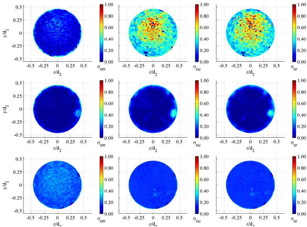
**Figure 6:** Contour plots of the standard deviation of the velocity components at the measurement plane upstream the fan for different inflow conditions: free inflow (top), HFC (middle) and TFC (bottom); standard deviation of the axial velocity (left), circumferential velocity (middle) and radial velocity (right).
