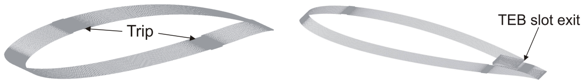
Figure 5. Numerical surface grid of the airfoil element; S834 reference (left) and TEB S834 (right).
