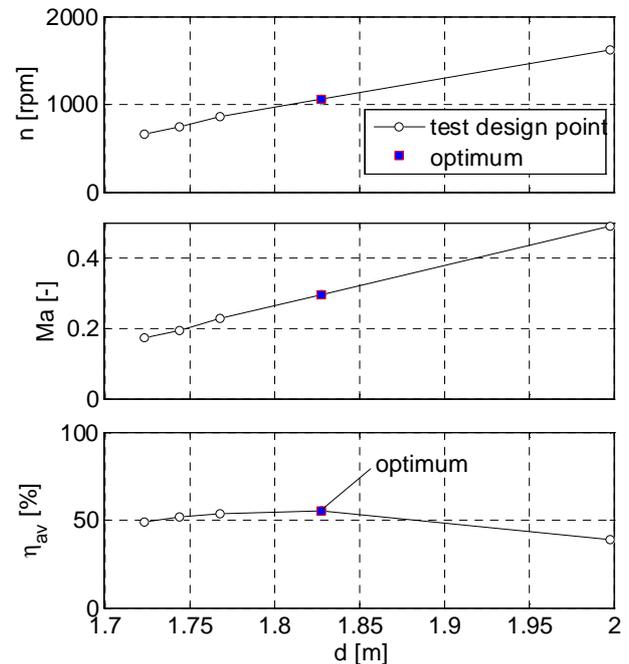
Fig. 7. Turbine D: Rotor diameter, rotational speed, circumferential Mach number and average efficiency for the five design points tested.
