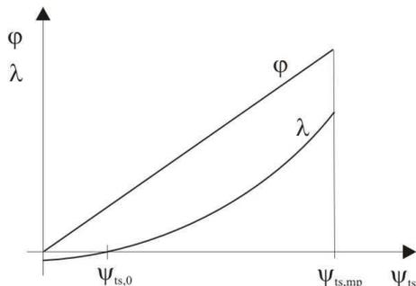
Fig. 2. Aerodynamic non-dimensional steady-state characteristics of a bidirectional turbine (schematically).
