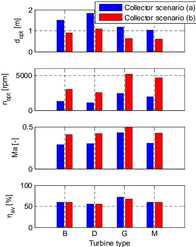
Fig. 10. All turbine types in the catalogue: Optimal parameters and average efficiency.
