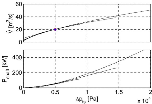
Fig. 5. Turbine D: Family of performance curves for the five design points tested; the marker corresponds to the available pneumatic power from the collector ('design' power).
