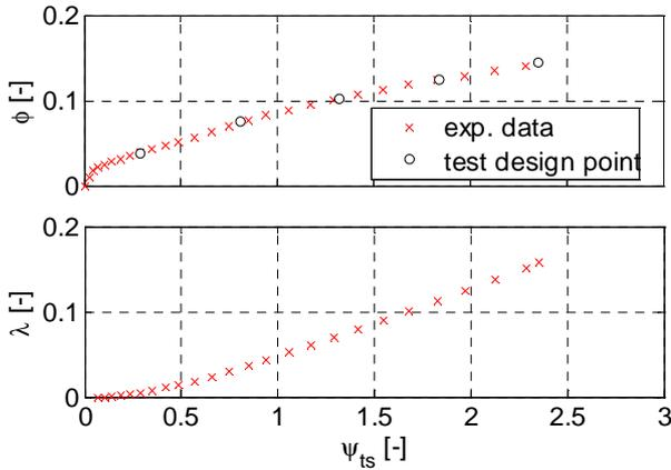
Fig. 4. Turbine D: Non-dimensional characteristics and five tested design points.
