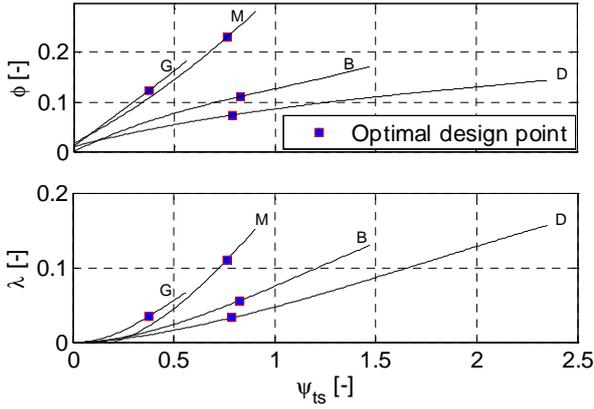
Fig. 8. Collector scenario (a) ('design' damping  $D_{ts} = 250 \text{ Pa}/(\text{m}^3/\text{s})$ ): Optimal design points for all turbine types in the catalogue.
