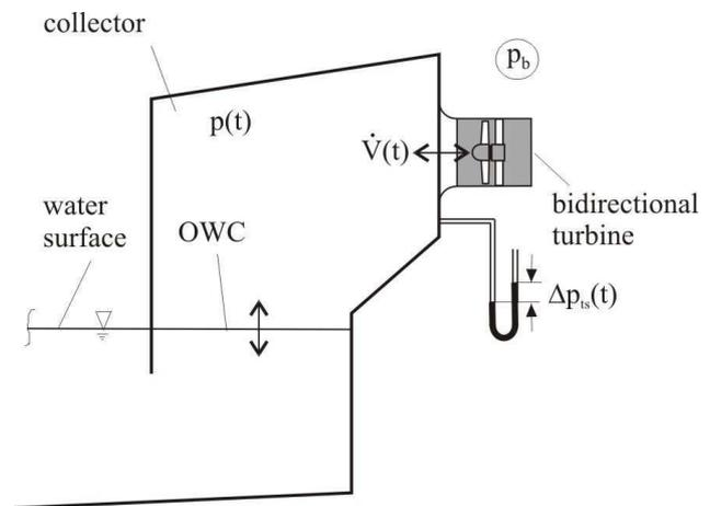
Fig. 1. Oscillating water column system (schematically).
