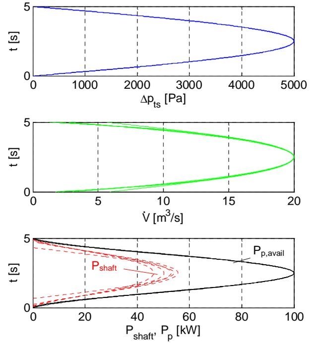
Fig. 6. Turbine D: Upper: Half cycle of pressure head input to the turbine; middle: volume flow rate through the turbine; lower: pneumatic power available from the collector and family of turbine shaft power according to the five design points tested.
