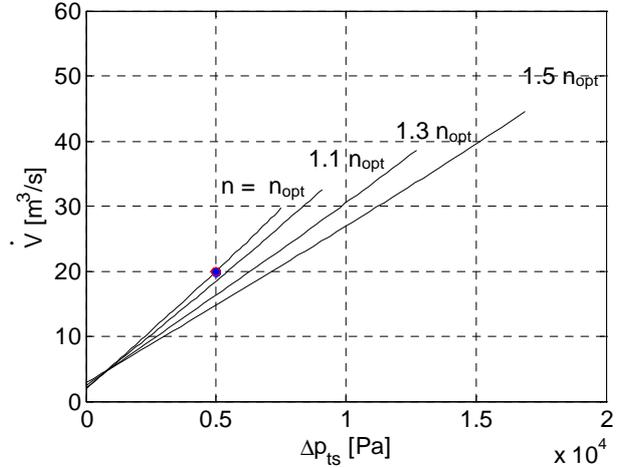
Fig. 11. Effect of the variation of rotational speed on performance curves (optimal turbine G for a 'design' damping  $D_{ts} = 250 \text{ Pa}/(\text{m}^3/\text{s})$ )
