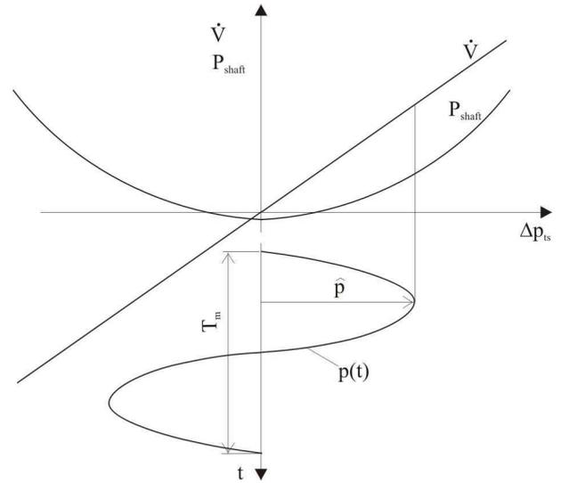
Fig. 3. Steady-state performance curves of a turbine with  $D$  and  $n = \text{const.}$  and sinusoidally varying pressure head (schematically).
