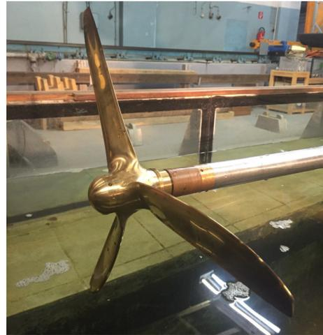
Fig. 6: 1:8 scaled brass model of the SCHOTTEL SIT250 for the validation experiments
