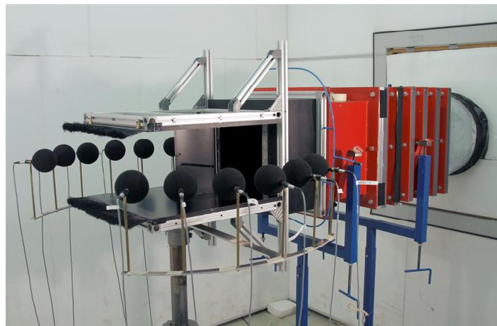
**Fig. C2:** Left: Schematic diagram of microphones around airfoil section (not to scale); right: Test rig and microphones in semi anechoic chamber
