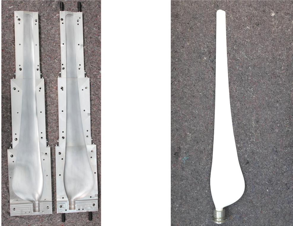
**Fig. 6:** The two halves of the mold and the new blade B-KV200
