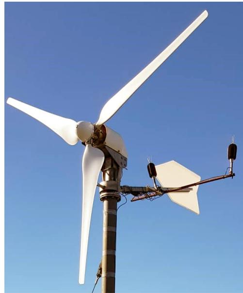
**Fig. A2:** Turbine mounted microphones (on-axis and one off-axis), left: schematic top-view diagram (not to scale)
