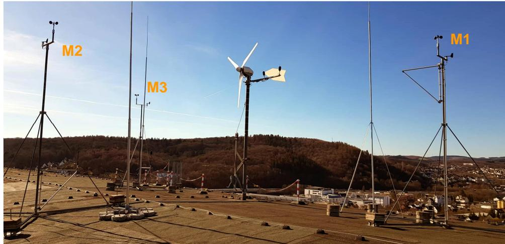
**Fig. A1:** Wind turbine and measurement stations M1, M2 and M3; each station is equipped with a cup anemometer and a wind vane type wind direction sensor
