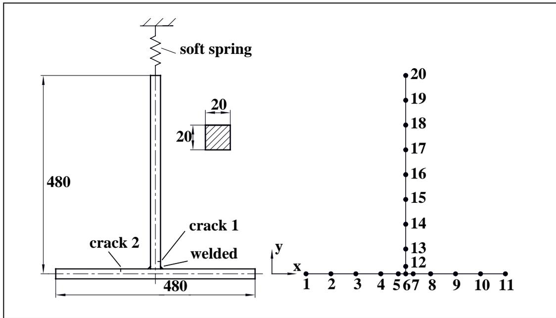
Figure 14: *Test structure and nodes of the FE model*
