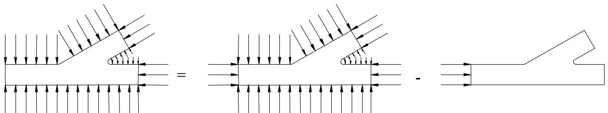
$$\vec{F}_{D_{M,2,3}} = - \int_{\substack{\text{Mantelfläche} \\ + A_2 + A_3}} p_a \vec{n} dA = - \underbrace{\int_{\substack{\text{Mantelfläche} \\ + A_1 + A_2 + A_3}} p_a \vec{n} dA}_{=0} - \left( - \int_{A_1} p_a \vec{n} dA \right)$$
