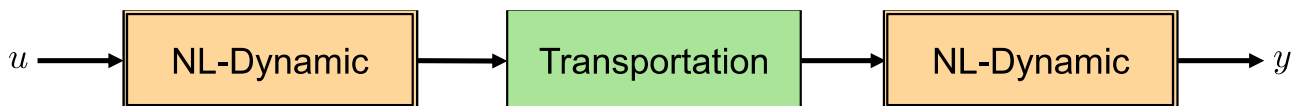
Figure 1: Block diagram of a nonlinear dynamic process with pure time delay in the transportation part
