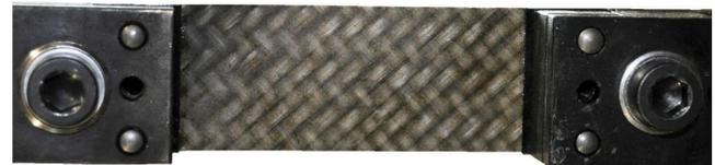
Figure: Clamping device with 36 mm specimen, undeformed configuration.
