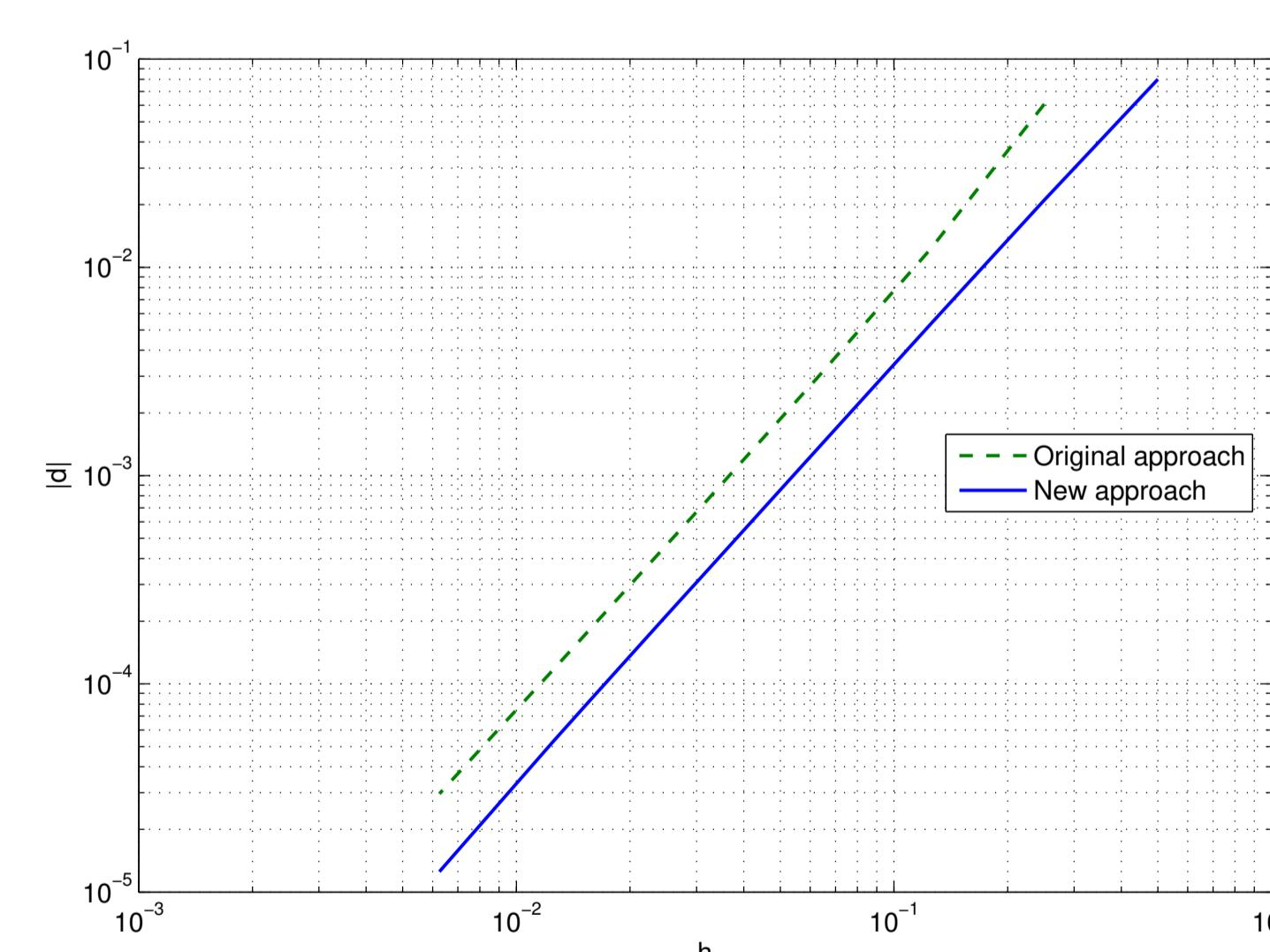
Errors in tip displacements versus h-refinement.
