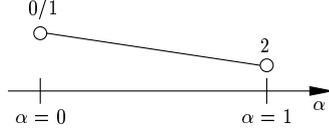
**Figure 3.1** Continuous polynomial approximation ( $k=1$ ) on the master element  $I_\alpha$ .
