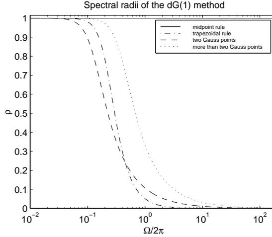
**Figure 4.3** Spectral radii of the  $dG(1)$  method associated with specific symmetric quadratures.
