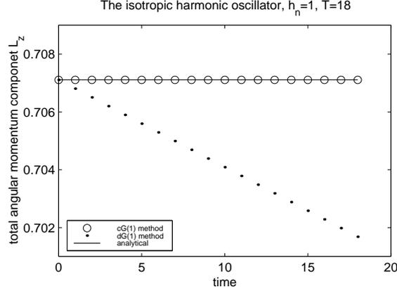
**Figure 4.4** The nonvanishing total angular momentum component  $L_\zeta = L_\zeta(t)$ , where the  $\zeta$ -axis is perpendicular to the plane of motion, of an isotropic harmonic oscillator with mass  $m=2$ , total energy  $H=0.25$  and potential constant  $c=-0.25$ . Computed with the cG(1) and dG(1) method with a time step size  $h_n=1$ .
