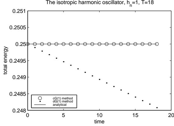
**Figure 4.1** Total energy  $H = \widehat{H}(t)$  of an isotropic harmonic oscillator with mass  $m=2$ , total energy  $H=0.25$  and potential constant  $c=-0.25$ . Computed with the cG(1) and dG(1) method with  $h_n=1$ .
