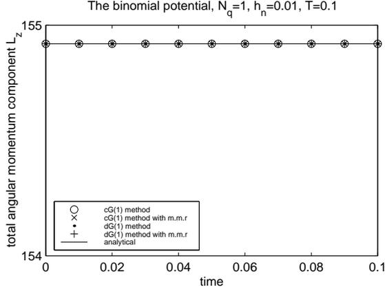
**Figure 4.7** The nonvanishing total angular momentum component  $L_\zeta = L_\zeta(t)$ , where the  $\zeta$ -axis is perpendicular to the plane of motion, of the potential  $V = \frac{1}{2} c (r^2 - 1)^2$  with mass  $m=2$ , total energy  $H=6000$  and potential constant  $c=1000$ . Computed with the cG(1) and dG(1) method associated with midpoint rule as well as modified midpoint rule (m.m.r). That is,  $N_q=1$ . The time step size  $h_n$  is 0.01.
