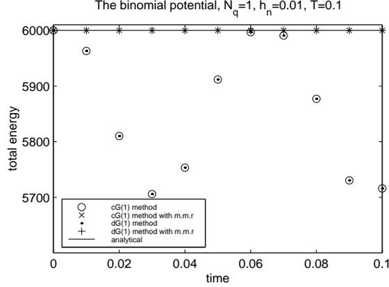
**Figure 4.6** Total energy  $H = H(t)$  of the potential  $V = \frac{1}{2} c (r^2 - 1)^2$  with mass  $m = 2$ , total energy  $H = 6000$  and potential constant  $c = 1000$ . Computed with the cG(1) and dG(1) method associated with midpoint rule as well as modified midpoint rule (m.m.r). That is,  $N_q = 1$ . The time step size  $h_n$  is 0.01.
