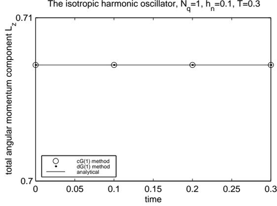
**Figure 4.5** The nonvanishing total angular momentum component  $L_\zeta = L_\zeta(t)$ , where the  $\zeta$ -axis is perpendicular to the plane of motion, of an isotropic harmonic oscillator with mass  $m=2$ , total energy  $H=0.25$  and potential constant  $c=-0.25$ . Computed with the cG(1) and dG(1) method associated with the midpoint rule ( $N_q=1$ ) and with a time step size  $h_n=0.1$ .
