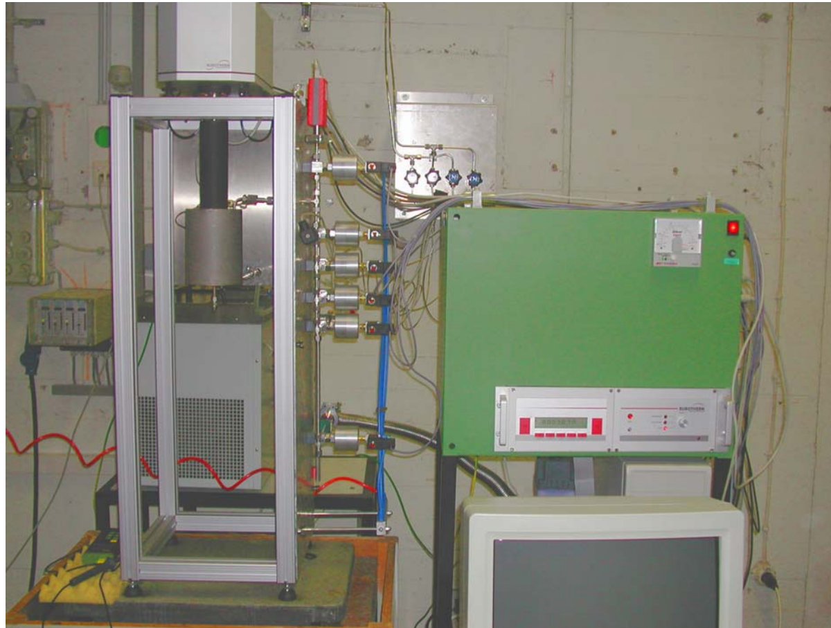
Automated MSB (2) (Rubotherm AG, Bochum) for Densimetric-Volumetric Measurements (DVMs) of binary coadsorption equilibria
