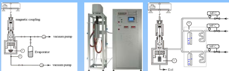
Fig. 2: Gravimetric system for measurement of vapor adsorption equilibria with static measuring method (left) or flow measurement method (right) on a magnetic suspension balance (center, Rubotherm).
