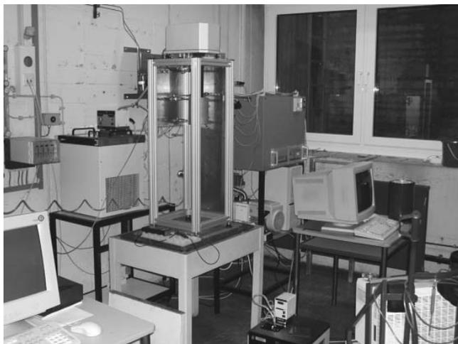
**Figure 2.** Instrument for volumetric–densimetric measurements of binary co-adsorption equilibria of gas mixtures on porous solids without using a gas chromatograph. The magnetic suspension balance, cf. Figure 1, near the centre is complemented by a thermostat at left, an electronic unit for automated measurements and control in the rear, a PC monitor at right and a helium gas-based instrument for leak detection in the foreground at right. © IFT University of Siegen, 2002.
