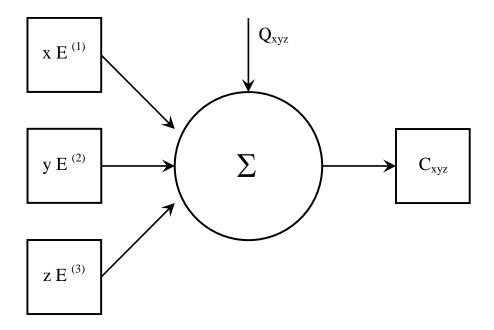
Fig. PH2. Ideal chemical reactor ( $\Sigma$ ) in which pure component ( $C_{xyz}$ ) is formed from pure chemical elements ( $E^{(1)}, E^{(2)}, E^{(3)}$ ) all substances being at standard states [PH4].
