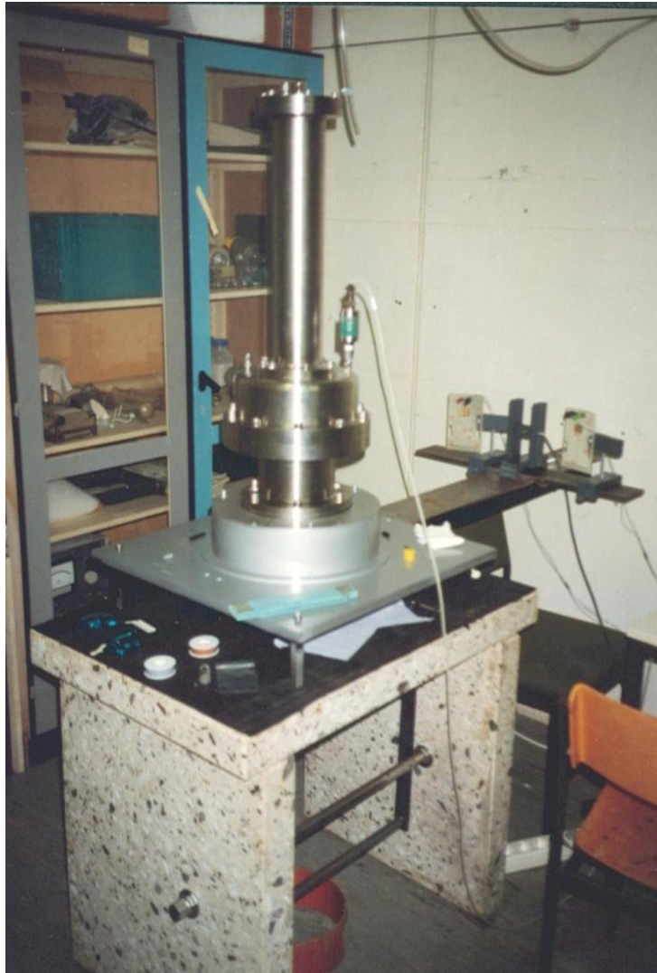
Rotational pendulum for measurements of gas adsorption equilibria by observing slow damped oscillations. Height of instrument: 1.5 m.
