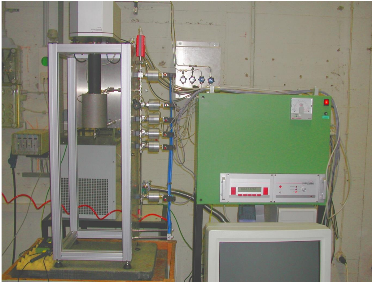
Automated MSB (2) (Rubotherm AG, Bochum) for DVMs of binary coadsorption equilibria
