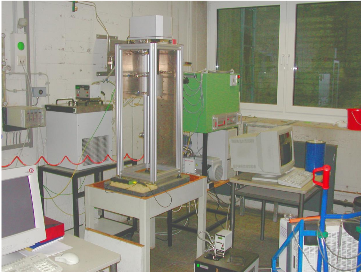
Instrument for DVMs of binary coadsorption equilibria using a MSB (2) (Rubotherm AG, Bochum)
